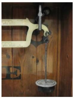
The pictures here show details of a Howe Scale console probably similar to the one at the King Store. It seems likely that the panel bearing the Howe Scale lettering, seen in the old King Store photo, was just a nameplate and that the scale was actually operated from the side opposite the platform, under the shelter of the porch roof, similar to the Fairbanks scale on the facing page.
